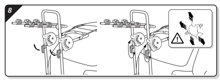
Ensure that both carrier clamping levers are in the closed position. Progressively tighten the levers on both sides of the carrier by turning them clockwise. When the resistance to turning starts to increase
